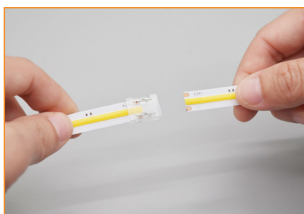
Put the LED strip directly into the connector and make sure both ends of led strip are tightly connected
