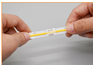
Make sure that the positive and negative match correctly, "+" to "+", "-" to "-"
