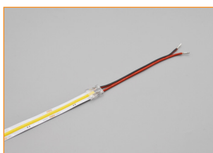
Make sure the positive and negative match correctly and press the sheet metal completely
